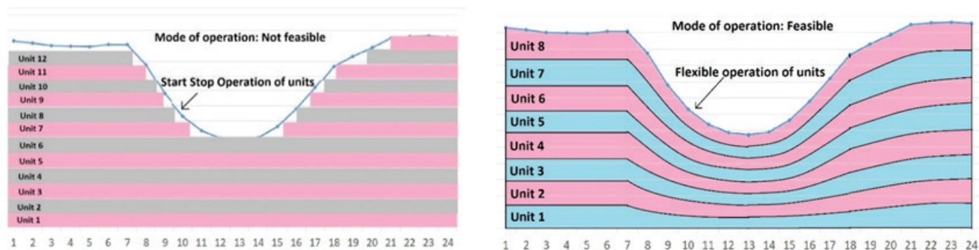
Figure 32 Mode of operation of thermal power plant
